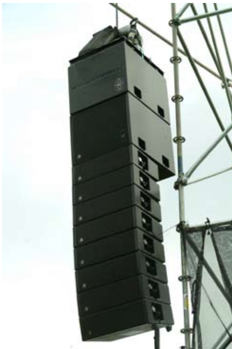
SpekTrix Subs flown in Cardioid with an underhang of 8 SpekTrix cabinets.
