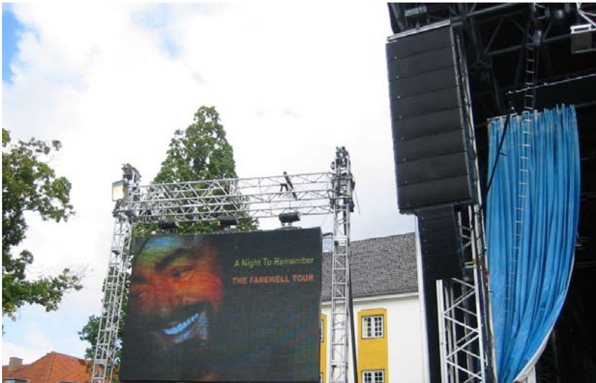
Y18 Flown with SpekTrix using Adamson Underhang kit.
